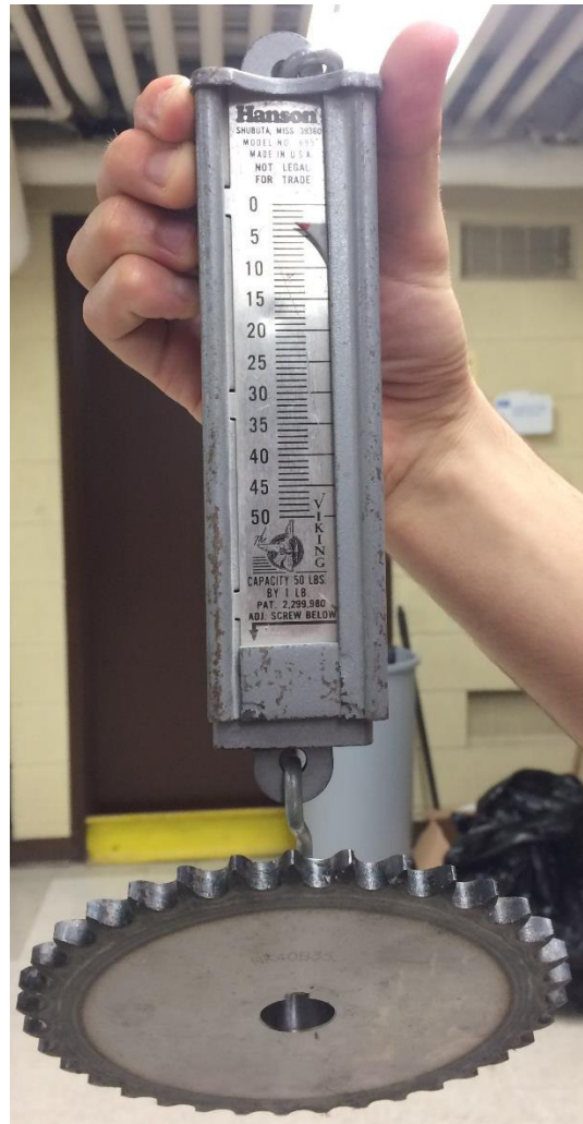
Figure 8. Measuring the sprocket weight
