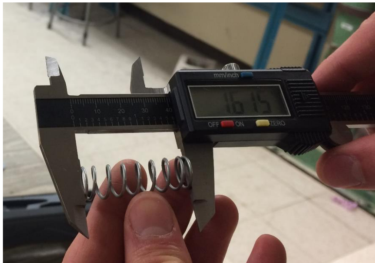
Figure 7. Measuring the spring length
