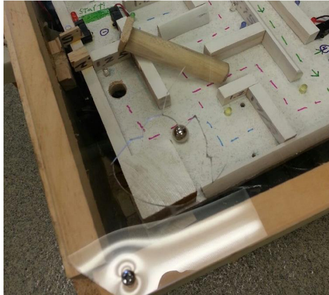
Figure 13. Compromised Plexiglas cover
